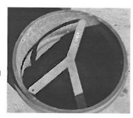
Step 2 Slowly lower the single leg of the gauge into the drum
